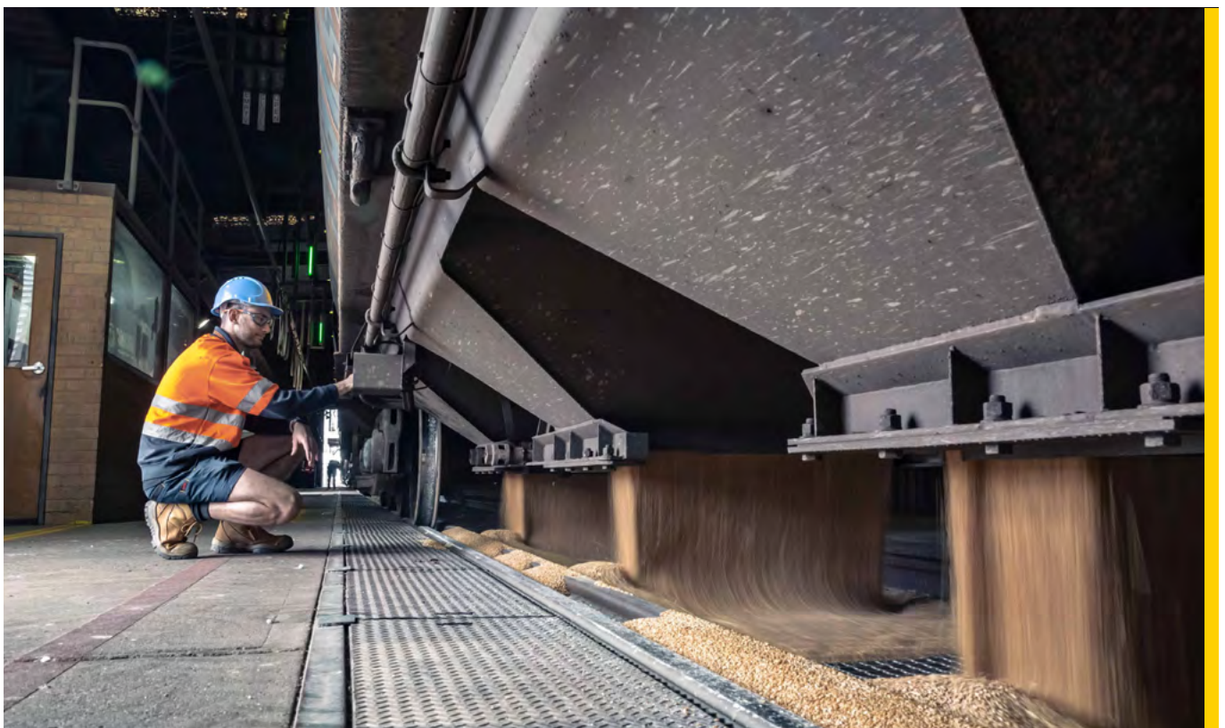
Unloading grain at our Carrington export terminal in Newcastle. Quality Assurance is a key factor in maintaining viable markets.
