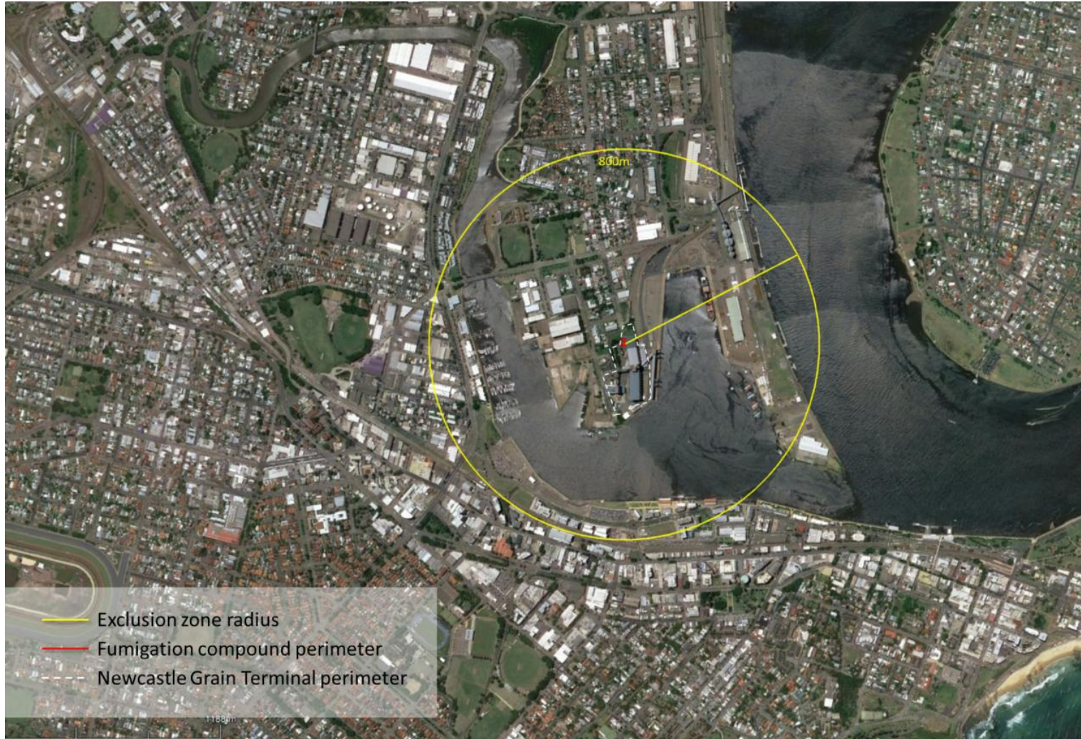
Figure 12 - Fumigation Incident - Major Leak Exclusion Zone
