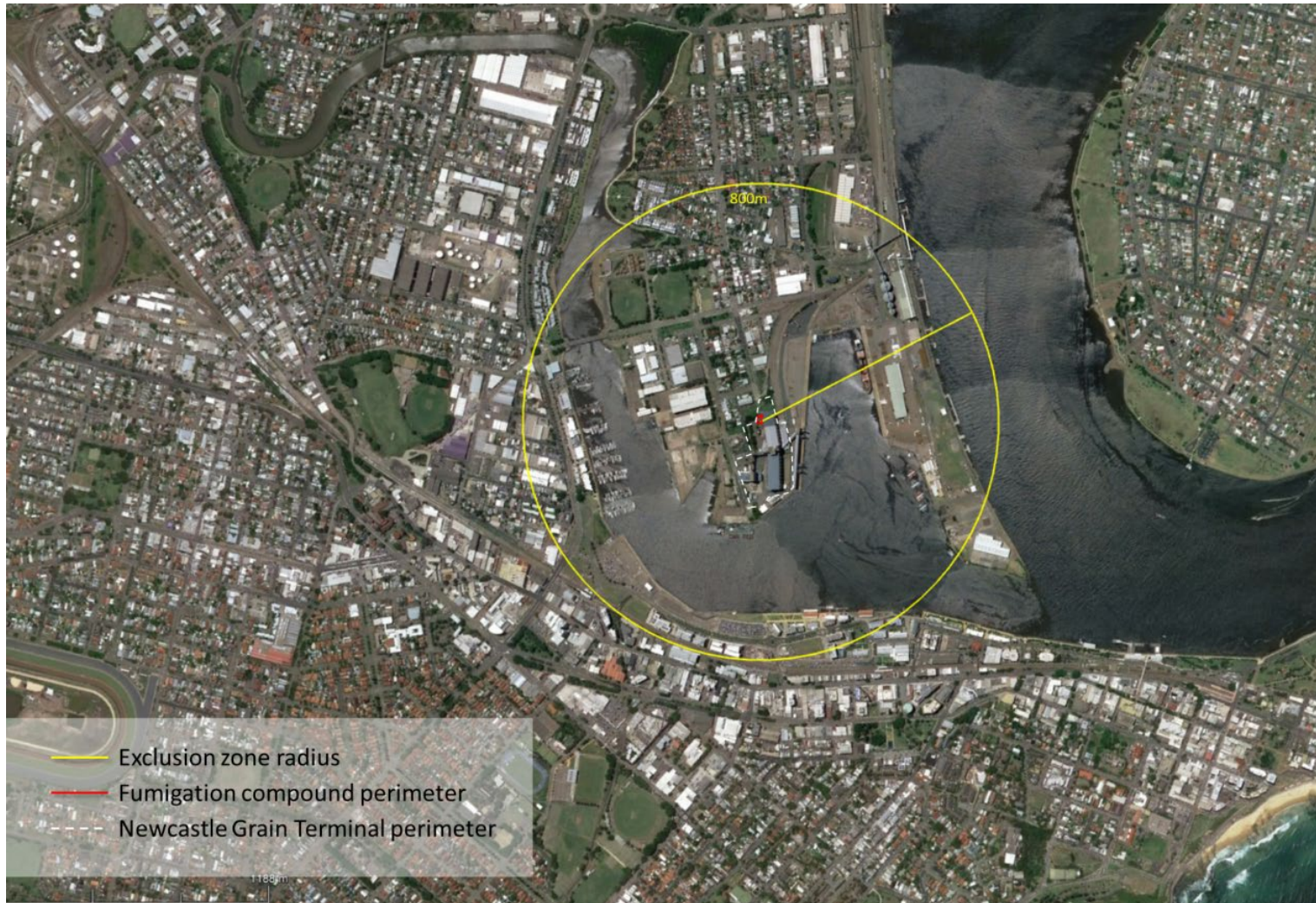
Figure 12 - Fumigation Incident - Major Leak Exclusion Zone
